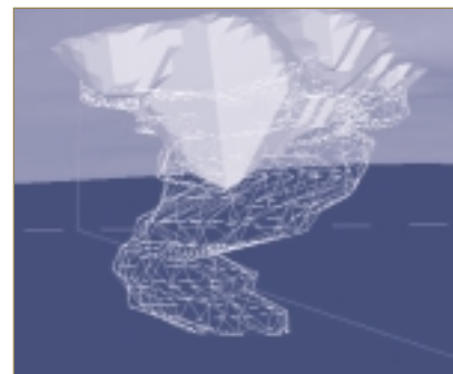
Alcaravan Open Pit and Wire Frame Outline of Resource Body (view up from subsurface to NE) 50 metres |-----|
